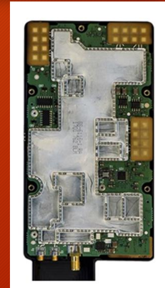
Early 5G Array Antenna Prototype with 3 x 8 element arrays (Qualcomm)
